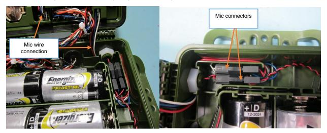
Next take both mic connectors out of the channel. With your index finger and thumb, grab both sides of the proper connector NOT THE WIRES and pull the connection apart while squeezing and wiggling the two parts of the connector.
